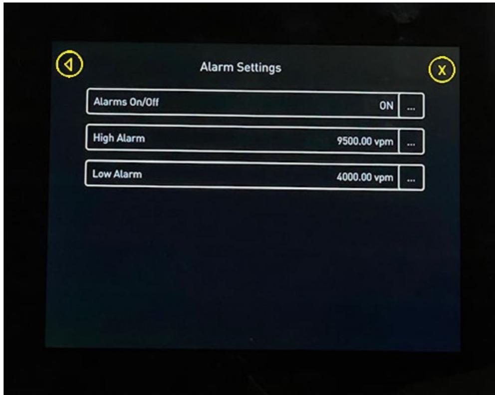
**8.1.1 ALARMS ON/OFF:** Ability to turn on or off set vibration alarms across the paving system.
