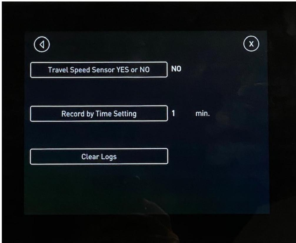
**13.1 TRAVEL (SPEED WHEEL):** If the system is equipped with a Travel Speed Wheel, this is where you turn that feature on.
